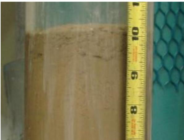
This control core, by comparison, shows no oil sediment.
